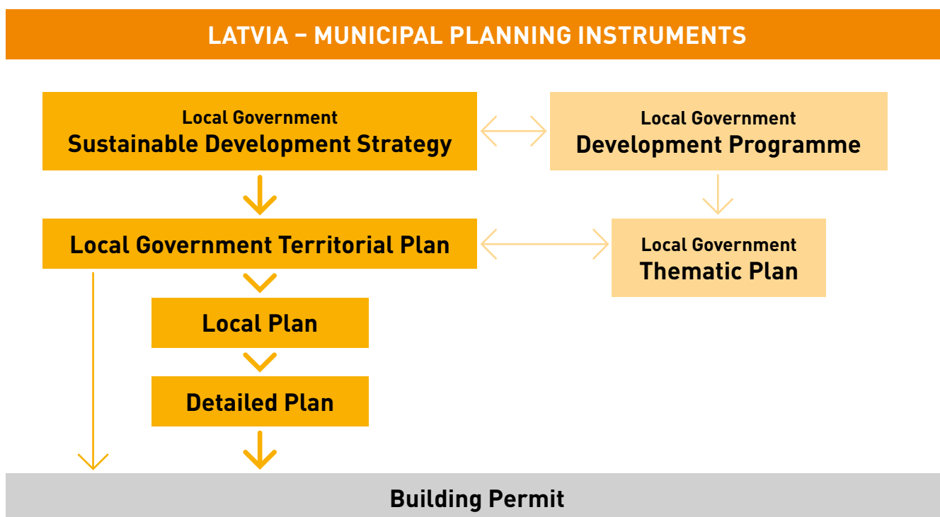
Figure 3. Planning instruments at the local level in Latvia (Source: Ministry of Environmental Protection and Regional Development)
